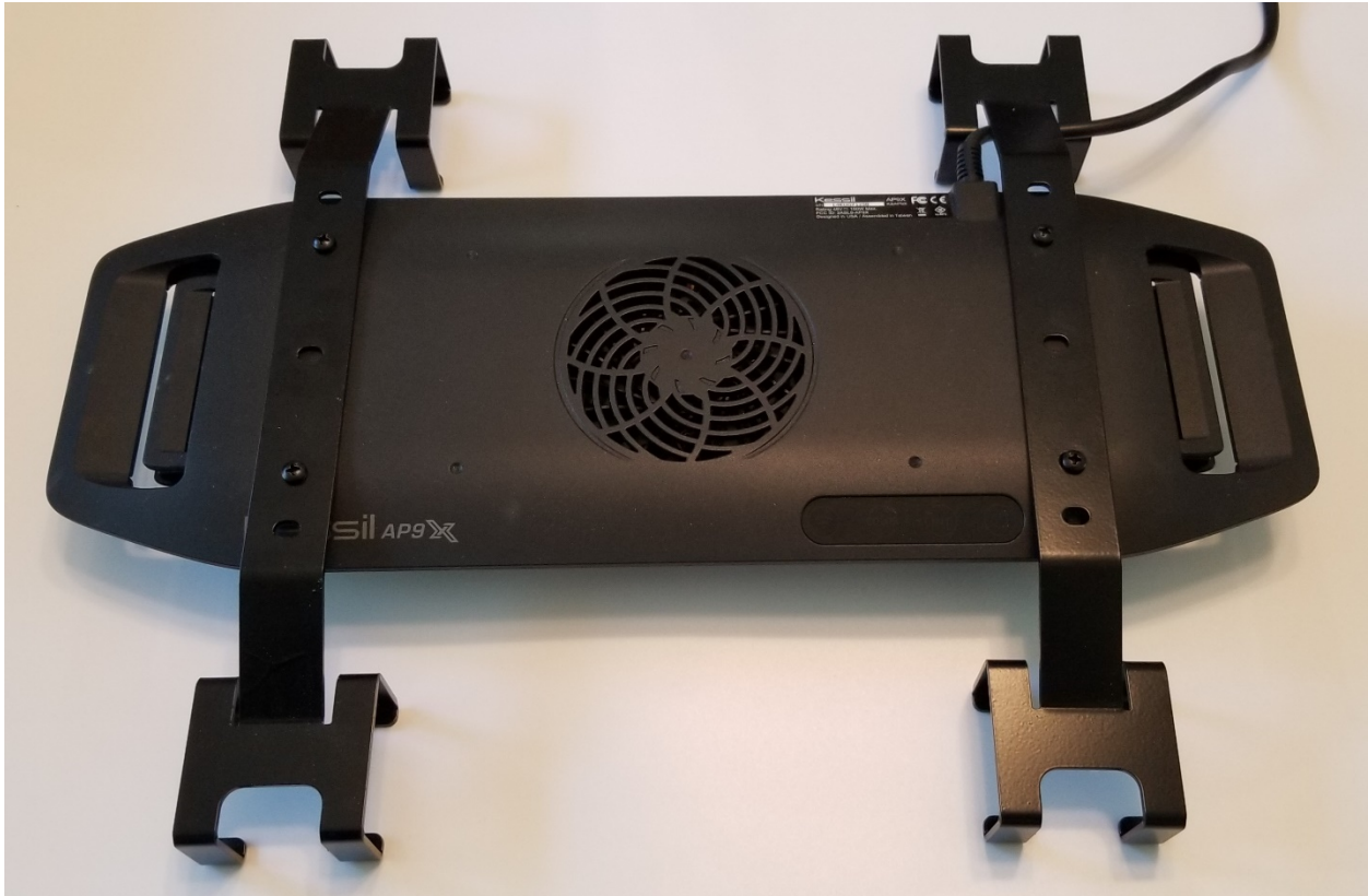
Figure 7 Light Brackets installed on AP9X
